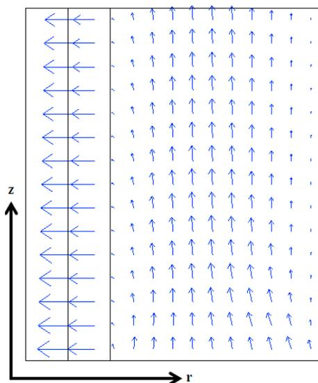
Figure 3. Arrows of total flux distribution of propylene in the contactor.
