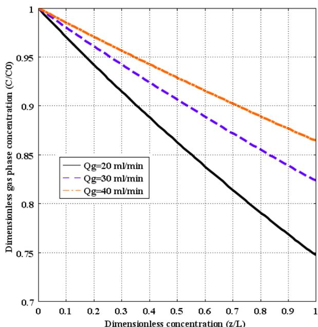
**Figure 8.** Dimensionless propylene concentration in the shell side along the length of the contactor at different gas-phase flow rates.
