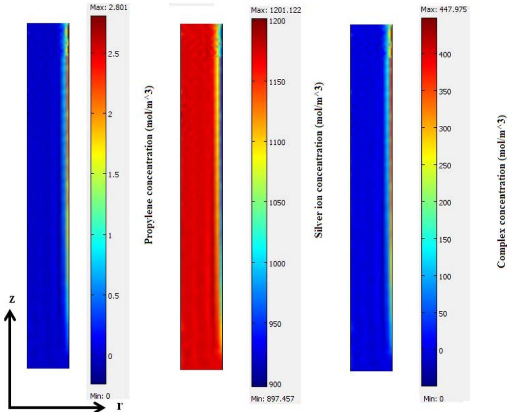
Figure 6. Concentration distribution of propylene, silver ion, and formed complex in the lumen side of membrane contactor.
