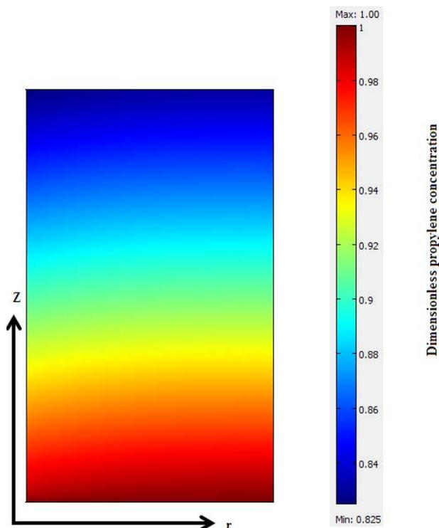
Figure 4. Dimensionless concentration distribution of propylene in the shell side of the contactor.
