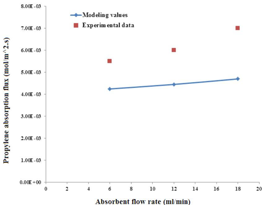
Figure 2. Propylene absorption flux vs absorbent flow rate for model validation.
