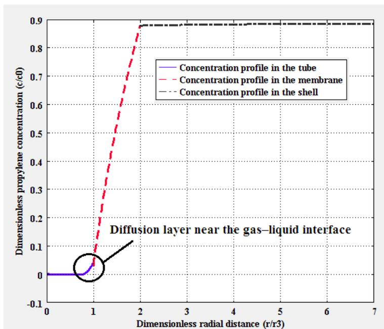
Figure 5. Propylene concentration profile in the radial direction at the middle of the membrane contactor ( $z/L = 0.5$ ).
