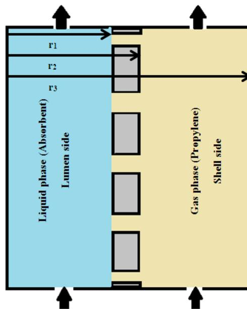
Figure 1. Cross-sectional area of the membrane contactor.
