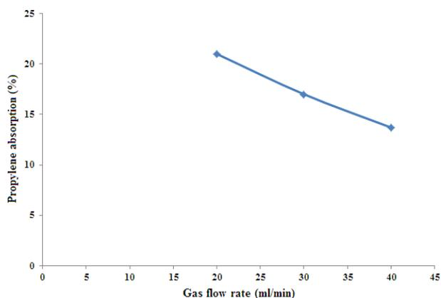
**Figure 7.** Effect of gas-phase flow rate in the shell side of the membrane contactor on propylene absorption efficiency.
